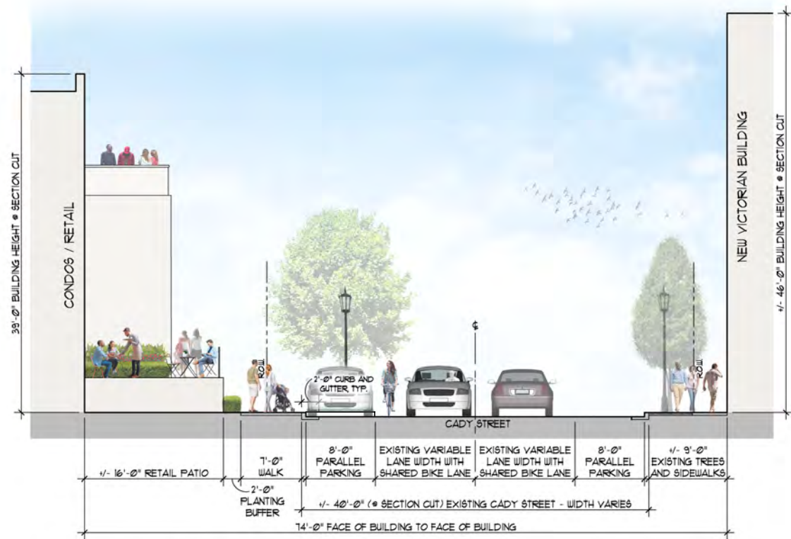
B Cady Street Cross Section (at condos and The New Victorian) SCALE: 1/8" = 1'-0"
